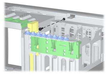
Figure 5-56 Installing the Front Bezel Security Screw
